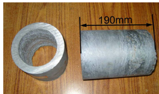
Fig. 1 Composite material tubes by centrifugal casting
